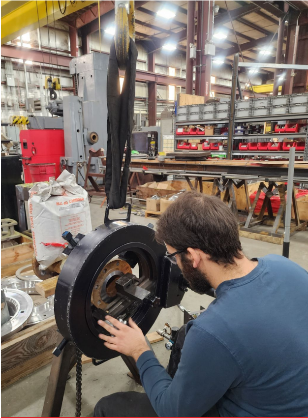
LA - Colby Roussel resurfacing a flange
